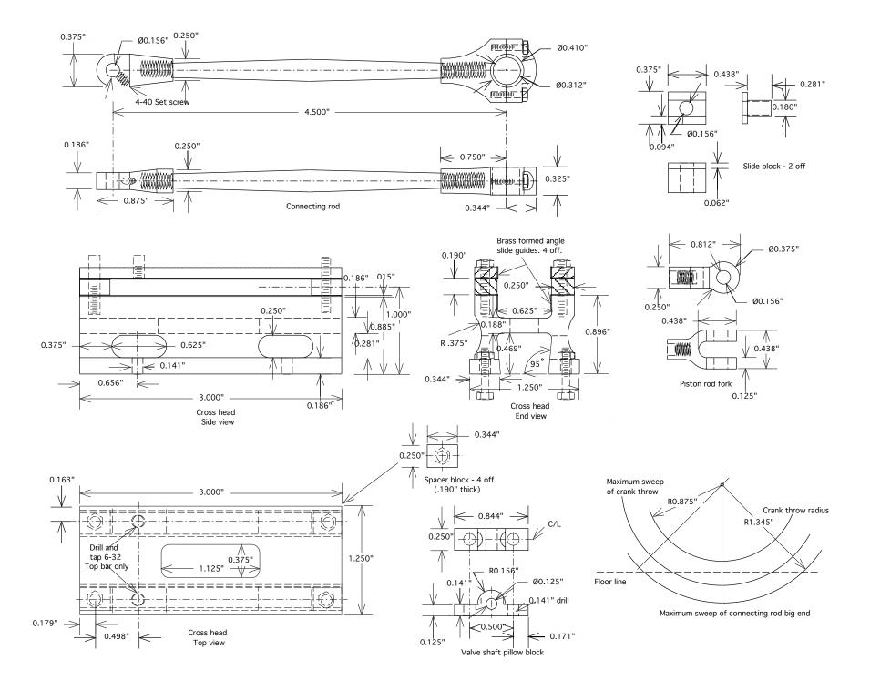
The connecting rod is shown at the top of the drawing. The crosshead slide block (of Two) is to the right. The crosshead is shown as side, end and top views. The pillow block (of two) for the valve bell-crank is shown at lower center. The crankshaft swing clearances are shown at the right.
